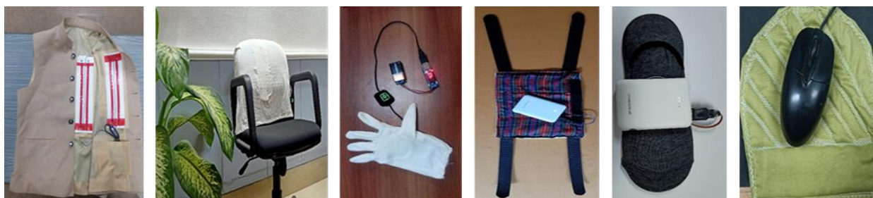
Figure 3. Heat generating textile products prepared using conductive yarn
